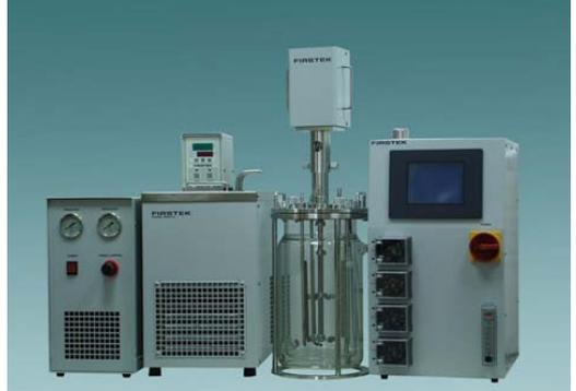
A 10-liter fermenter system consisting of a central stainless steel bioreactor with a stirrer, connected to various control units and sensors. The system is set against a light blue background.                                                                                                          |
